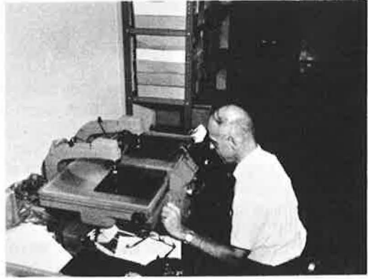
Wild PUG-3 point transfer device used for marking points on the diapositives.
