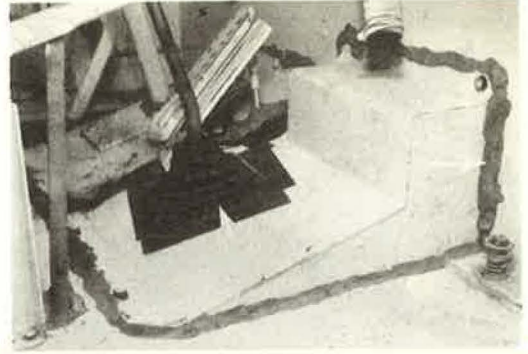
Figure 8. Sealing between cab and engine.
