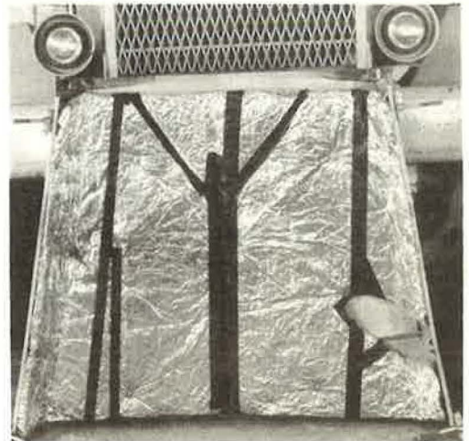
Figure 10. Foil-covered fiberglass hood liner.
