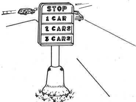
Figure 8. Suggested ramp control signal for multi-vehicle metering.
