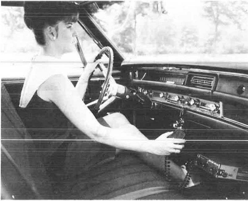
Figure 3. Typical CB radio (transceiver) mobile installation.
