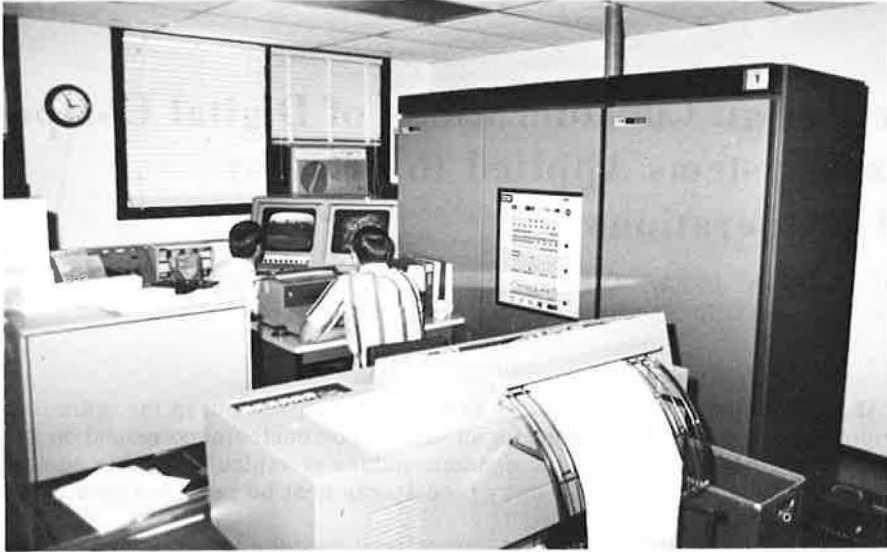
Figure 11. Digital computer data acquisition and control system in the Gulf Freeway Surveillance and Control Office.
