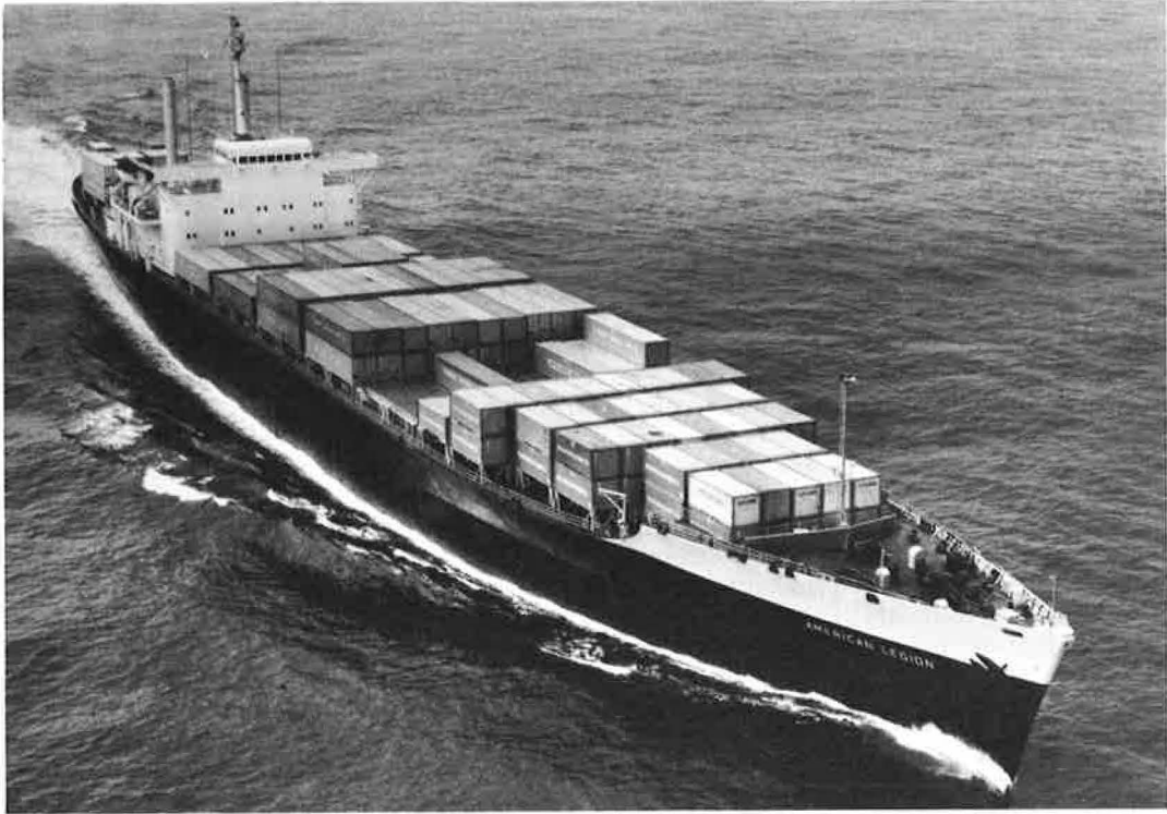
Figure 3. U.S. Lines high-speed containership carries both 20- and 40-ft containers.
