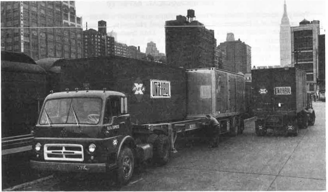
Figure 2. Steadman system side-shifter moves containers between railcar and trailer.
