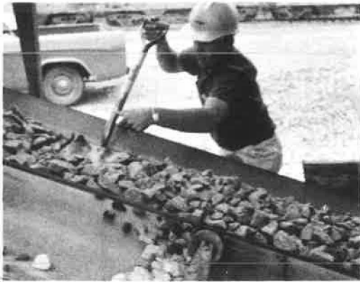
Figure 3. Sampling from a stopped belt.
