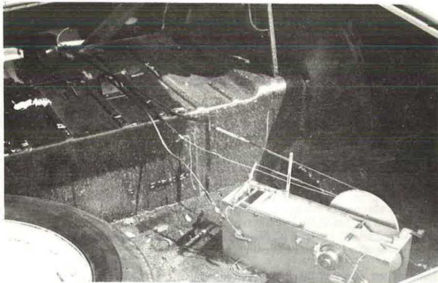
Figure 1. The Mays Road Meter installed in trunk compartment of automobile. Note the three cables leading to the left. The top cable is connected to the differential housing; the center cable leads to the front seat and is the on-off control; and the lower cable, which also leads to the front seat, is the event marker control.
