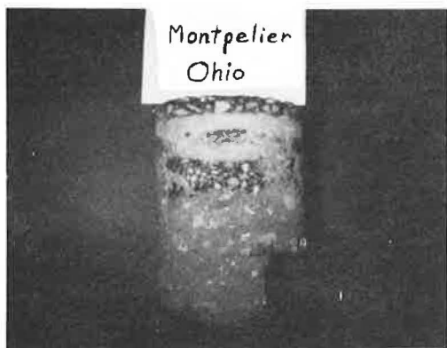
Figure 3. Salt-stabilized core from Montpelier, Ohio.
