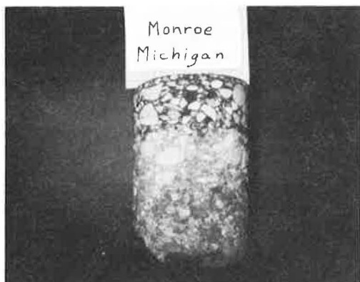
Figure 1. Salt-stabilized core from Monroe, Michigan.
