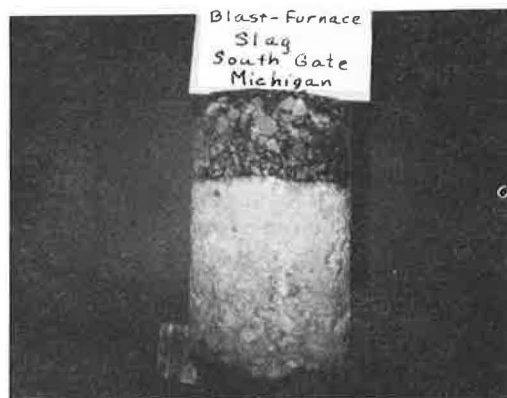
Figure 4. Salt-stabilized core composed of blast-furnace slag from South Gate, Michigan.
