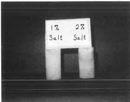
Figure 7. Two synthetic cores, one containing 1 percent salt and the other containing 2 percent salt, after being subjected to 30 cycles in the cycling apparatus.
