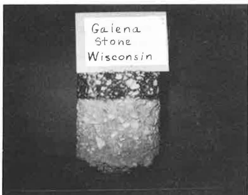
Figure 5. Salt-stabilized core of galena stone from Wisconsin.
