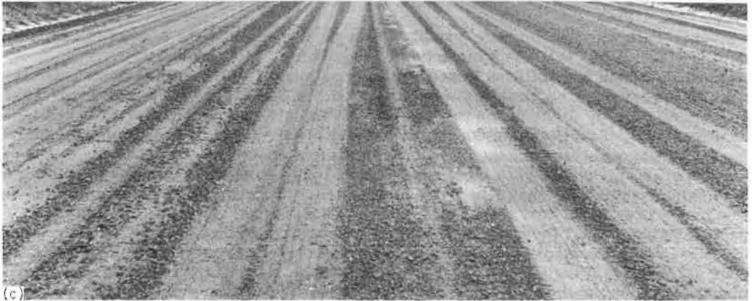
Figure 5. Typical test sections prior to application of prime coat: (a) 12 percent fines; (b) 9 percent fines; (c) 5 percent fines.
