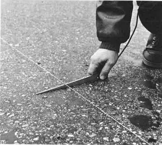
Figure 11. Rutting measurement device: (a) general view of unit and (b) depth indicator.
