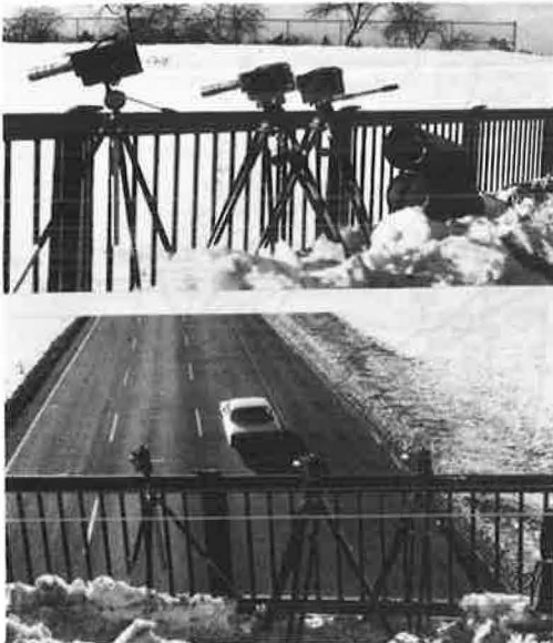
Figure 4. Position of cameras on overpass structure.
