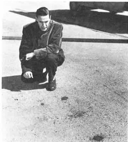
Figure 4. Installations of the ice-sensor units in the bridge deck surfaces.
