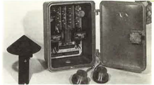
Figure 6. Control center and sensor units for the new dual-channel detection system for frost, snow, and ice on highway overpasses and bridges.
