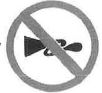
Figure 14. Sign indicating prohibition of use of audible warning devices.
