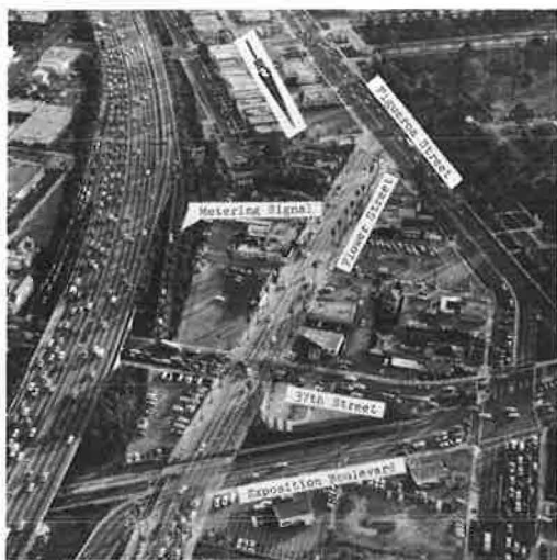
Figure 6. 37th Street on-ramp where platoon metering is used because of high metering rates used. Most traffic comes from southbound Flower Street and is stored in the left-turn lane upstream of Exposition Boulevard. Left turns to the ramp from westbound 37th Street are prohibited because they would interfere with eastbound 37th Street traffic. Right lane of the ramp is striped and signed for buses and emergency parking only. Congestion in northbound lanes is the result of a previous incident in the northbound lanes and is not affecting southbound traffic at this time.
