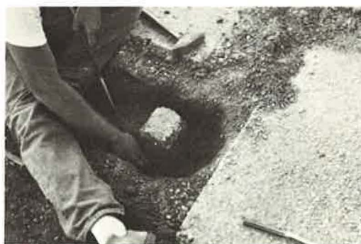
Figure 11. Synthetic flexible bases sampled for laboratory testing after several years of service in the Houston area.
