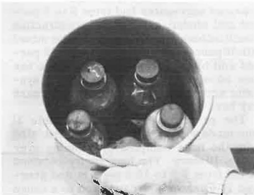
Figure 13. Container designed to fit shaker for agitating 5 samples simultaneously.
