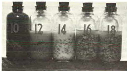
Figure 8. Complete samples immediately after cooking and subsequent agitation in water (numbers refer to approximate firing temperature, hundreds of degrees F).
