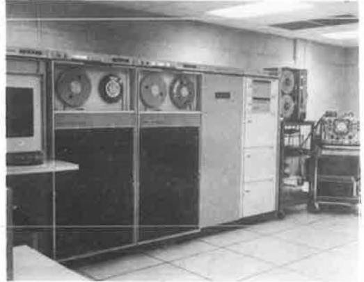
Figure 9. SDS 930 computer console and equipment hookup for A-D processing.
