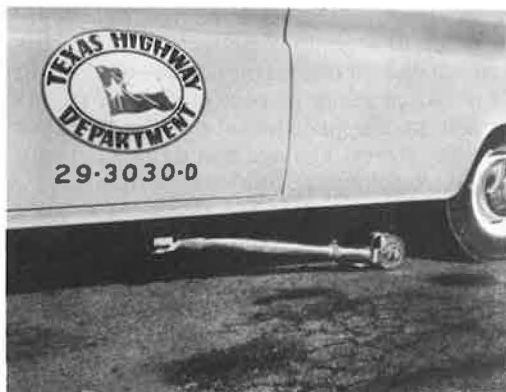
Figure 5. Road-following wheel and assembly.
