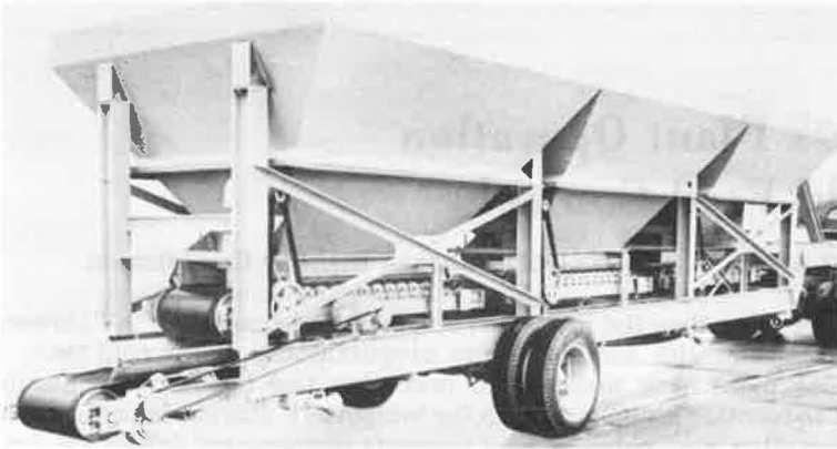
Figure 1. Cold feed blending plant.
