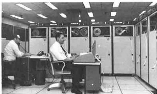
Figure 1. The Pennsylvania Department of Highways utilizes 2 Burroughs B5500 computers in the central office Data Processing Center. A portion of the operation is shown here.
