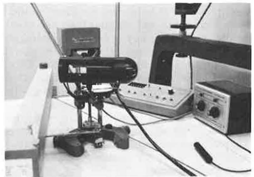
Figure 6. A close-up view of the horizontal scaler, operator control panel, and the stereo-image alternator system.
