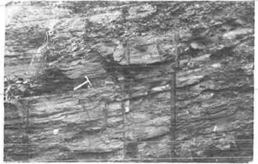
Figure 8. Offset boreholes in shale and siltstone intersected by road cut. Sliding of plates along bedding planes is toward observer in direction of dip of strata with lower plate having moved relatively more than upper.
