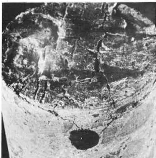
Figure 7. Core through incipient surface spall.
