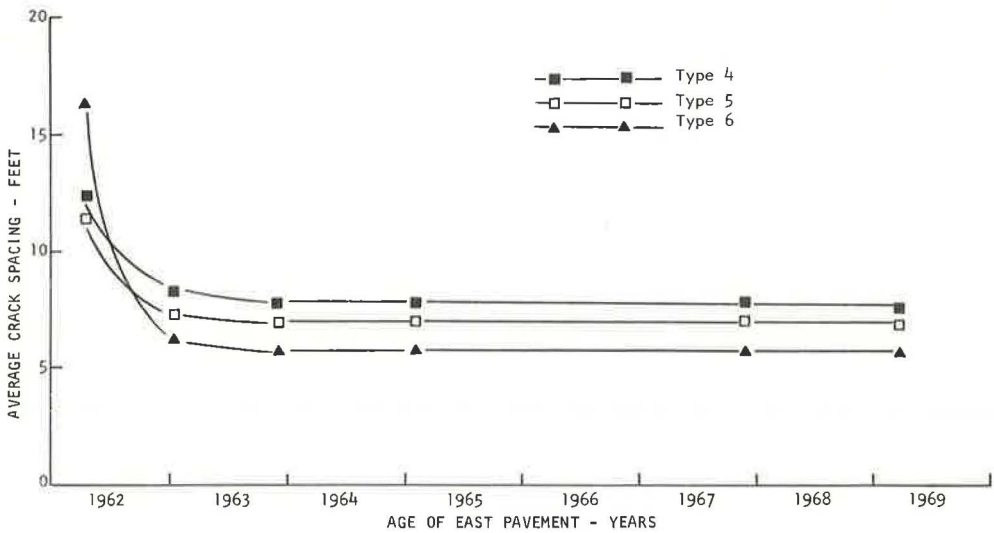
Figure 12. Average crack spacing of pavement with wire reinforcement on east roadway in Jones County.
