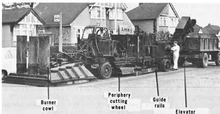
Figure 10. Special machine used to remove a given layer of bituminous pavement.
