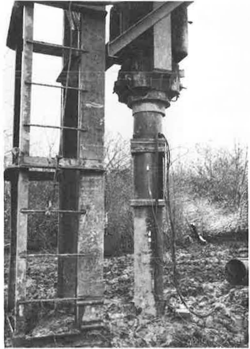
Figure 5. Force transducer and accelerometer in driving system.
