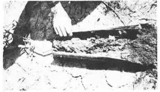
Figure 2. Sequence of soil textures ranged from a coarse sand at the top of the tube to a fine silt loam at the bottom to stimulate deep root development.
