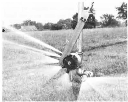
Figure 17. Rotary valve, adjustable swath, nozzle assembly equipped with rack and pinion, with rack operated by push-pull cable.
