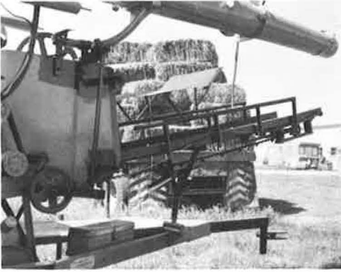
Figure 5. First version of mechanical feed table for delivering baled straw to mulcher.
