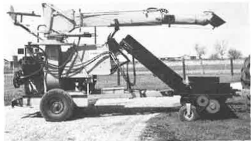
Figure 8. Finn straw mulcher with modifications for applying corncob mulch.
