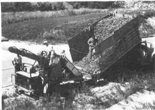
Figure 11. Mulcher with revised hopper and elevator for unbaled mulches.
