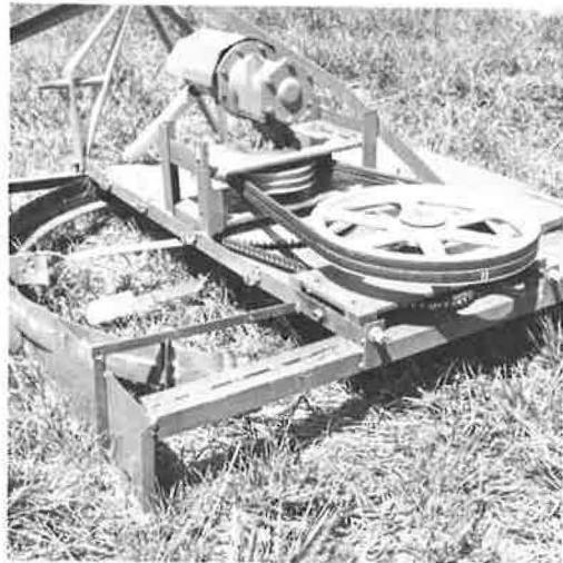
Figure 13. Shelf discharge mower with part of case removed; paddles move one-quarter the knife speed.
