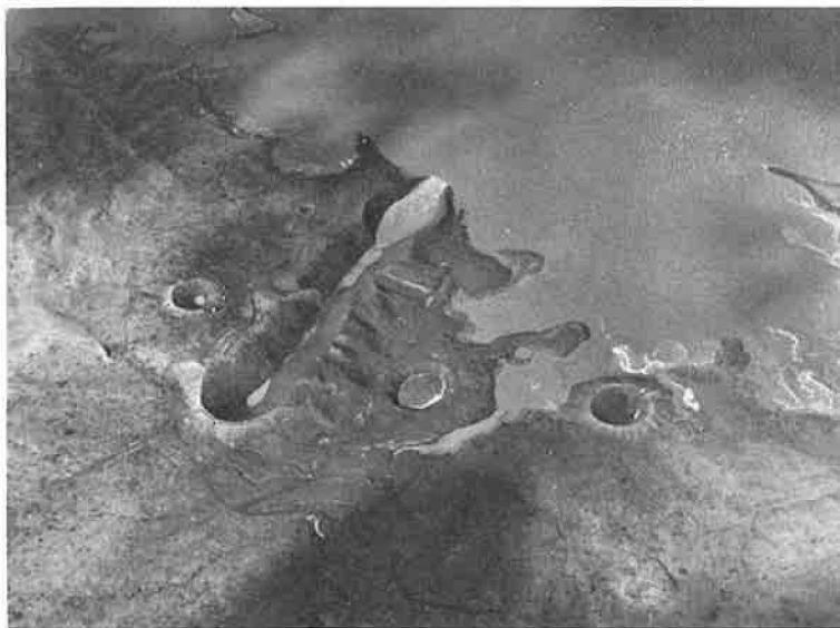
Figure 6. Reservoir connection experiment crater immediately following the detonation, showing water starting to fill the crater.
