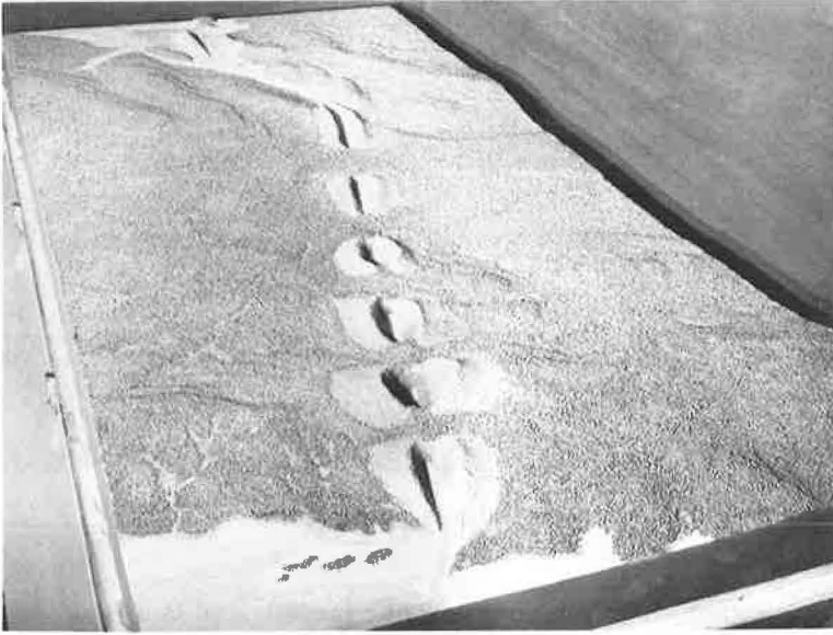
Figure 19. Model of transisthmian sea-level canal nuclear excavation showing results of first-pass detonations.
