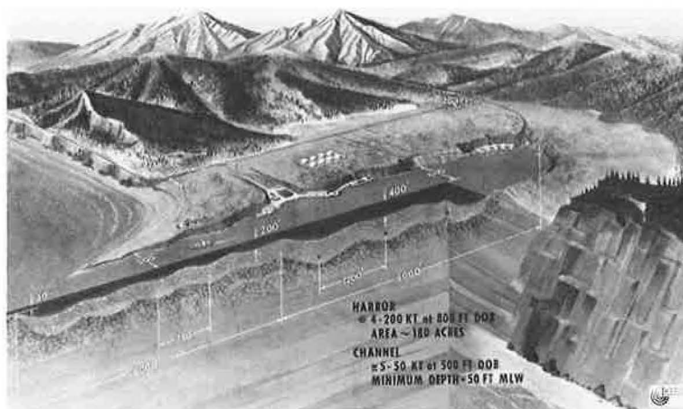
Figure 17. Harbor excavation concept.
