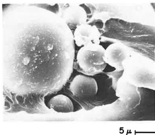
Figure 14. Fracture surface of a 10 percent by volume A-1100 treated glass bead-PPO composite.
