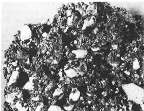
Figure 2. Laboratory-duplicated specimen showing stripping after freeze-thaw cyclic test.
