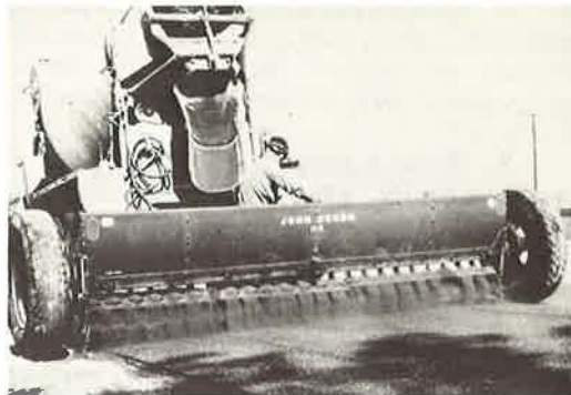
Figure 28. Seeder used for spreading pre-coated sand leaves ridges.
