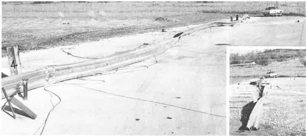
(c) View from vehicle approach (see insert for overall view from upstream)
