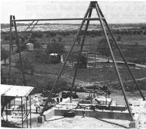
Figure 1. Southwest Research Institute pendulum impact tester.
