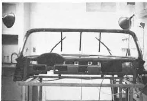
Figure 1. Apparatus used in evaluations of windshield cleaning implements and cleaning agents.
