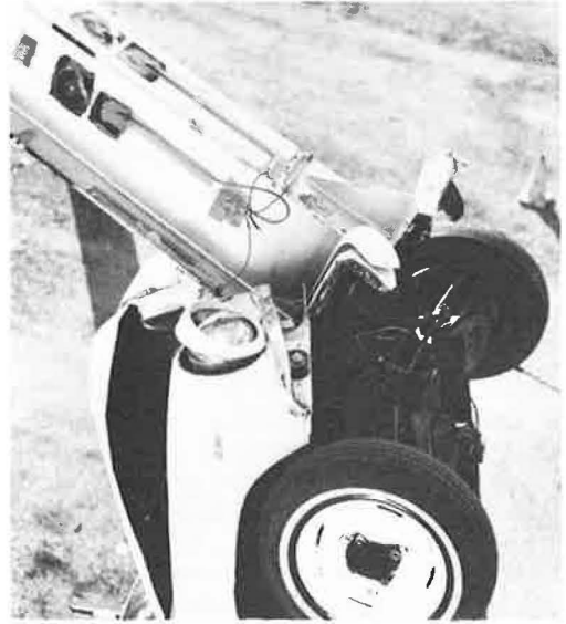
Figure 10. Vehicle wedged between support and ground (Test B).
