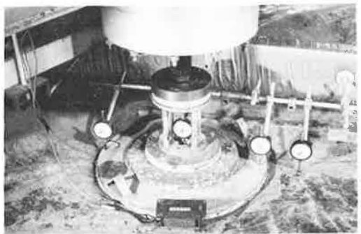
Figure 3. Close-up view of loading plate and gage system.
