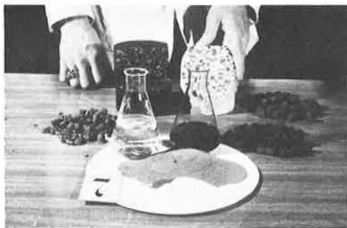
Figure 2. Fly ash and clay mixtures, fired pellets, and finished products using fly ash aggregate.
