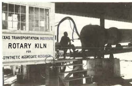
Figure 1. Pilot rotary kiln at Texas A&M University.
