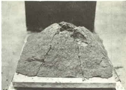
Figure 6. Failure surface for 2.8-bell diameter spacing.
