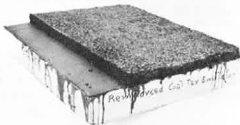
Figure 7. Laboratory test of bridge deck coating on 3- by 18- by 24-in. concrete block.
