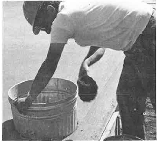
Figure 9. Sampling procedure for particle size analysis.
