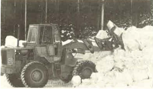
Figure 1. Articulated wheel loader equipped with a reversible one-way plow.
