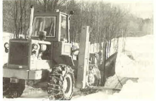
Figure 2. Articulated wheel loader equipped with vee plow and wing.
