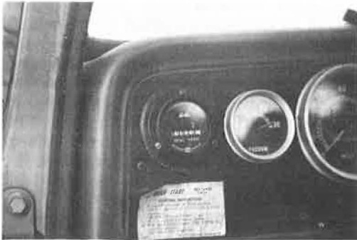
Figure 5. Hobbs hour meter mounting.
