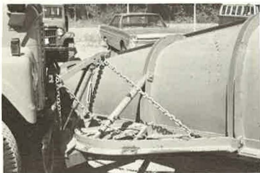
Figure 3. Washington standard moldboard with chain and turnbuckle assembly.
