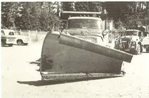
Figure 2. Washington standard power reversible moldboard with rubber snowplow blade.
