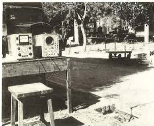
Figure 9. General setup of experiment, with amplifier and recording oscilloscope assembly shown on left.
