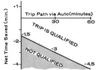
Figure 7. A criterion for deciding whether an automobile trip would save enough time to qualify for further synthesis processing.
