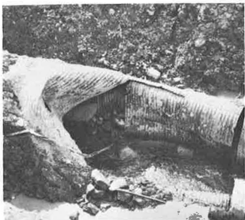
Figure 13. Complete collapse of 96-in. pipe.
