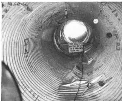
Figure 10. Pipe wall buckled at invert in dense soil (this is exceptional, for buckling is usually between 10 and 2 o'clock).
