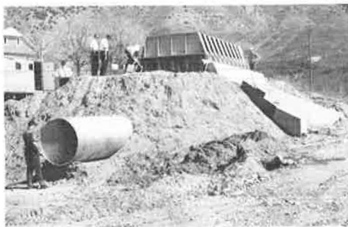
Figure 4. Loading beams being lowered into position where they are pinned before load is applied to cell (top), and test cell loaded and ready for test to begin (bottom).
