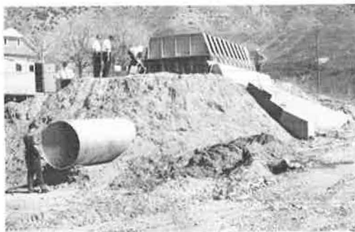
Figure 4. Loading beams being lowered into position where they are pinned before load is applied to cell (top), and test cell loaded and ready for test to begin (bottom).
