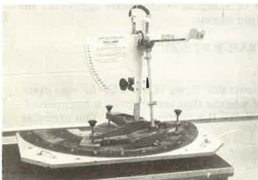
Figure 3. British portable skid-resistance tester.
