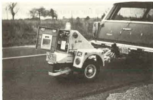
Figure 1. Mu-meter friction trailer.
