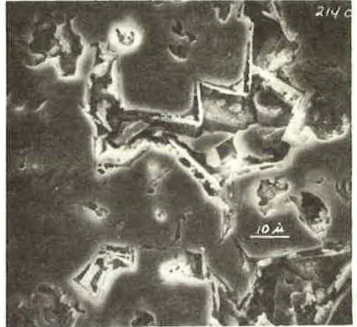
Figure 5. Electron micrograph of rejection texture showing clay plates around dolomite crystals, polished and etched in 0.1 normal HCL.
