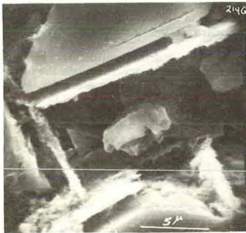
Figure 6. Electron micrograph of rejection texture showing clay plates around dolomite crystals.
