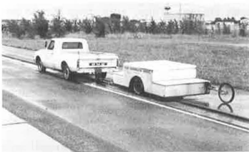
Figure 3. Tow truck and instrumented test trailer.
