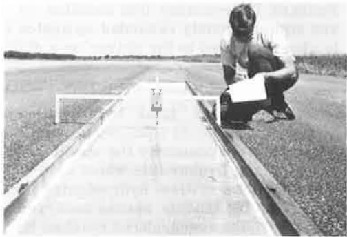
Figure 2. Typical water depth reading taken before test on hydroplaning trough.
