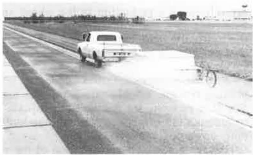
Figure 4. Typical test run on hydroplaning trough.
