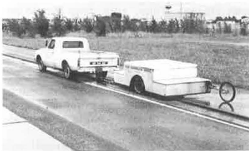
Figure 3. Tow truck and instrumented test trailer.
