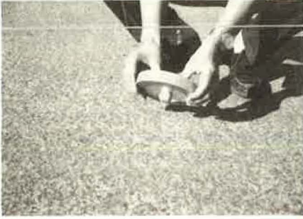
Figure 7. Putty impression method for measuring surface macrotexture.
