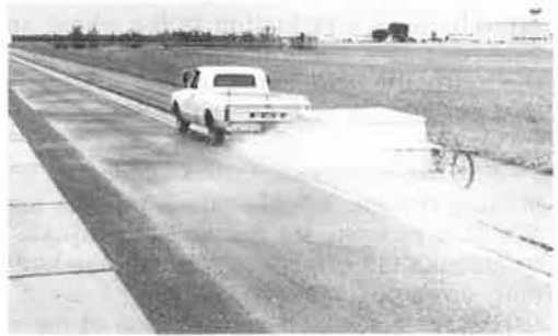
Figure 4. Typical test run on hydroplaning trough.
