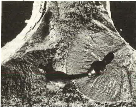
Figure 4. Two small fatigue cracks that initiated from pores in the longitudinal fillet weld and grew perpendicular to the axis of the weld (~x5.5).
