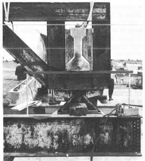
Figure 5. Testing frame showing scales used to determine rotational displacements of end of specimen.
