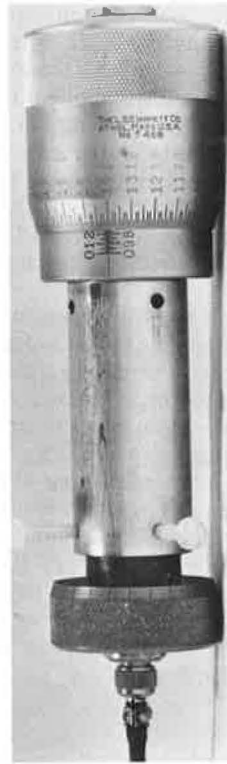
Figure 10. Micrometer and jig for calibrating UC-3 transducers.
