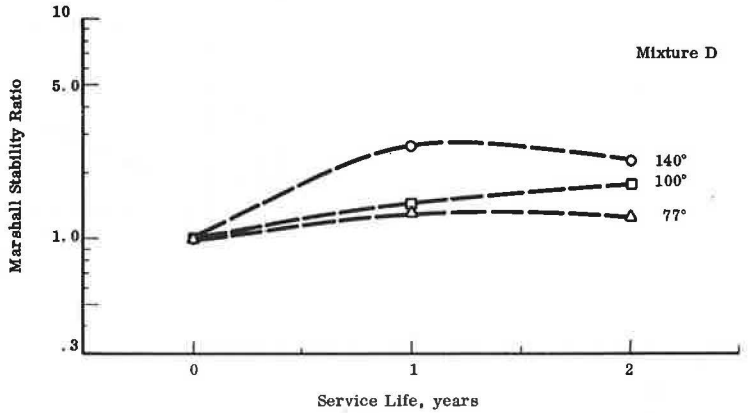
Figure 4. Age dependency of Marshall stability, mixture D.
