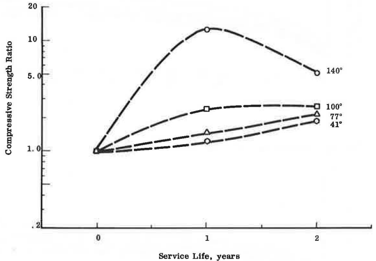
Figure 5. Age dependency of compressive strength, mixture D.
