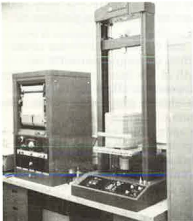
Figure 3. Loading and recording equipment for cone penetrometer test.
