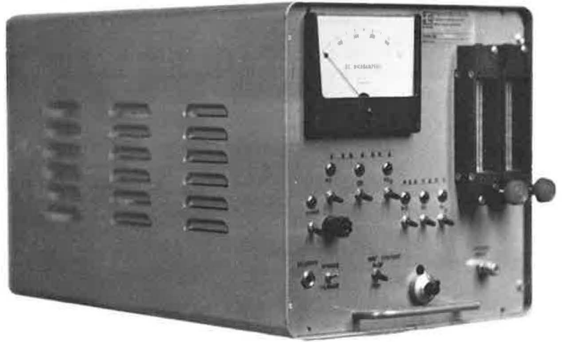
Figure 3. Breadboard instrument for monitoring automobile exhaust pollutants.
