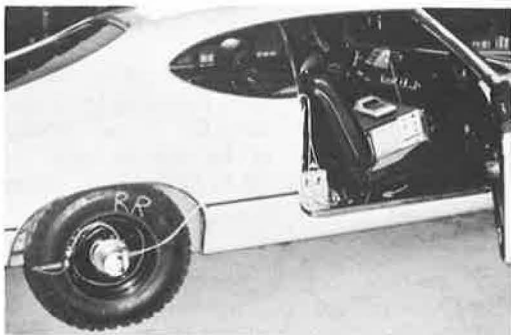
Figure 20. Test equipment used for dynamic-force measurements.
