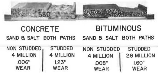
Figure 10. Pavement sections worn after laboratory test.
